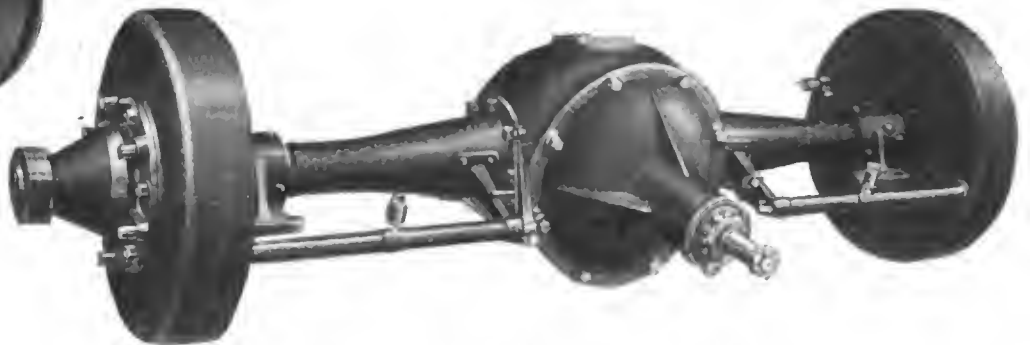
Semi-floating rear axle with single brake drums used on the Fageol chassis
